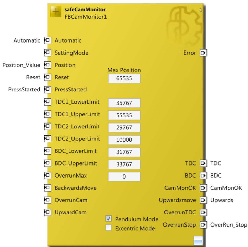
Figure 3-110: Function block CAMMONITOR
