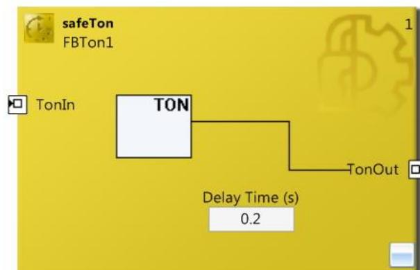
Figure 3-56: FB TON in TwinCAT 3
